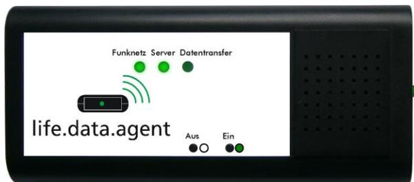
6. The next step is the **transmission of your health data**. The Life Data Agent transmits all data automatically. This process is indicated by the **third LED** (right).
