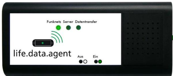
5. Blinking of the **second LED** (middle) shows that the **connection to the data base** is in progress. The LED stay lighted when the connection to the data base is established.
