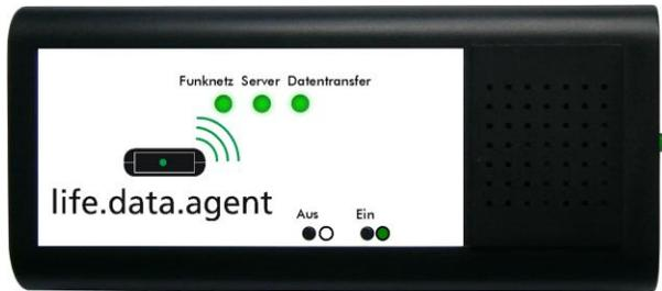
7. As soon as all data are transmitted successfully **all three LED** are switched on permanently. A few seconds later the Life Data Agent switches off automatically.
