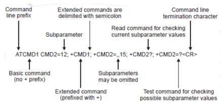
Figure 3-2: Basic Structure of a Command Line
