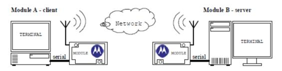
Setup the PDP context AT+CGDCONT=1,"IP","apn","0.0.0.0",0,0 OK Create MIP Call (activate PDP context) context) AT+MIPCALL=1,1,1 OK +MIPCALL: 1,1,"172.16.157.52 socket AT+MIPOPEN=1,1,1020,"172.16.80.103",1010,1
