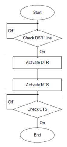
Figure 5-2: RS232 Lines Setup
