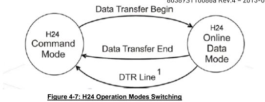
Note: <sup>1</sup>AT&D settings = 2 or 3. The operation closes the actual FTP connection and switches H24 to command mode.
