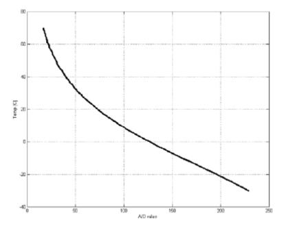
Figure 4-9: Temperature vs. A/D Value
