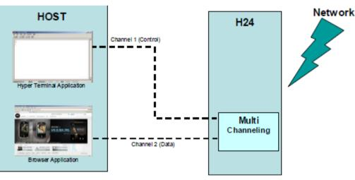
Figure 2-5: H24 with Multi Channel Support Capabilities
