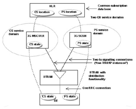
Figure 2-3: Class A Mode of Operation
