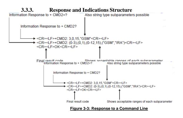
If verbose responses are enabled (using the command V1) and all the commands in a command line have been performed successfully, the result code  $\langle CR \rangle \langle LF \rangle OK \langle CR \rangle \langle LF \rangle$  is sent from the H24 to the terminal. If numeric responses are enabled (using the command V0), the result code  $0 \langle CR \rangle$  is sent instead.
