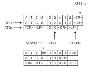
Figure 3-4: Flow and Structure Configuration Commands
