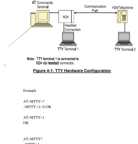
Figure 4-1: TTY Hardware Configurationshows the TTY hardware configuration.
