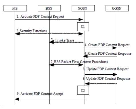
Figure 2-4: PDP Context Activation Diagram Originated by H24
