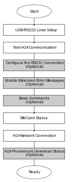
Figure 5-1: Recommended H24 Initialization Workflow
